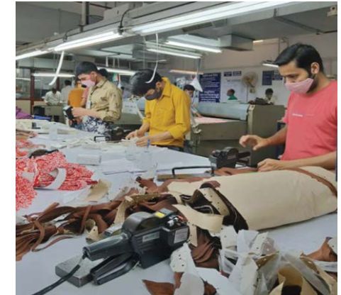
Ticketing of cut garment – Repetitive work; requires checking / adjusting unique number on the ticketing machine (accessible interface missing), good hand dexterity must
