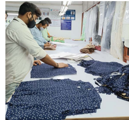
Bundling of cut garments – Repetitive work; requires standing for hours, layering cloth (seem by seem), bunding and numbering as per ticketing sequence
