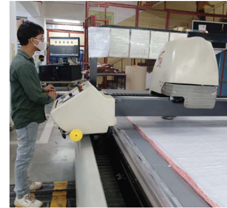
Layering and Cutting Function – requires standing for hours, layering cloth (seem by seem), viewing Auto-Cad drawings and monitoring cutting as per template
